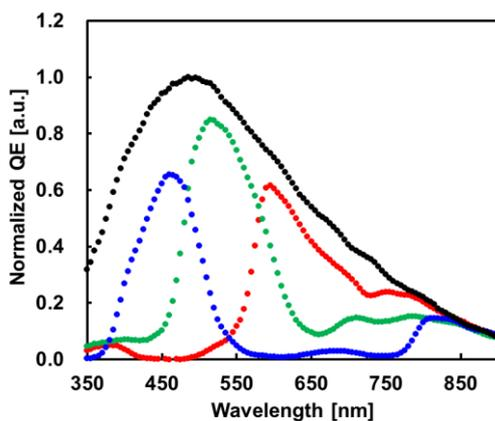
**Fig. 5. QE spectrum of red, green, blue, and white pixel**
