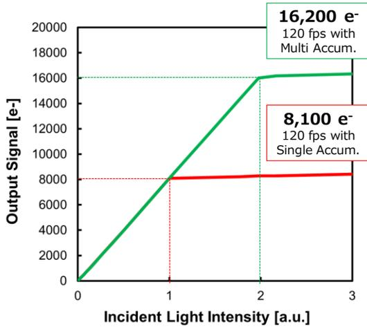
**Fig. 4. Measured output characteristics**
