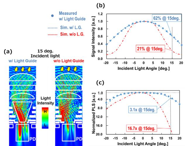
**Fig. 7. (a) Simulation of the light intensity profile, (b) incident light angle dependence of sensitivity, and (c) PLS**
