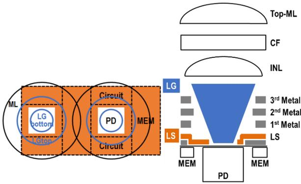
Fig. 2. (a)Layout and (b) cross section diagram of LS and LG structure
