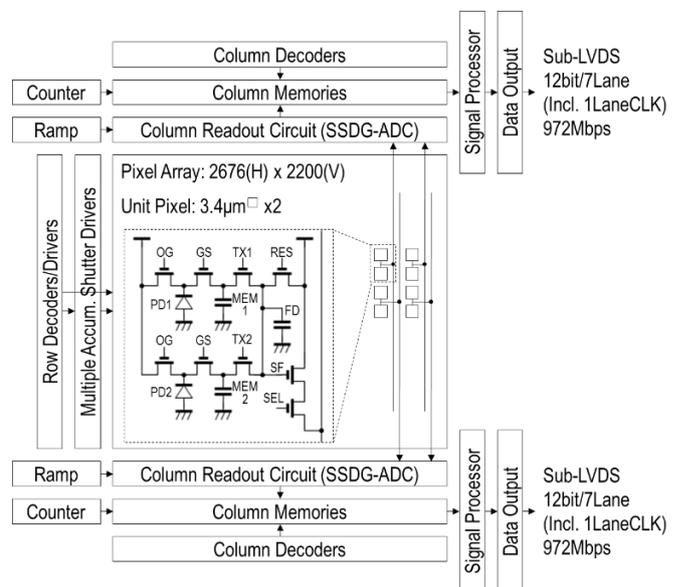
**Fig. 1. Block diagram of the GS CIS and pixel circuit schematic**
